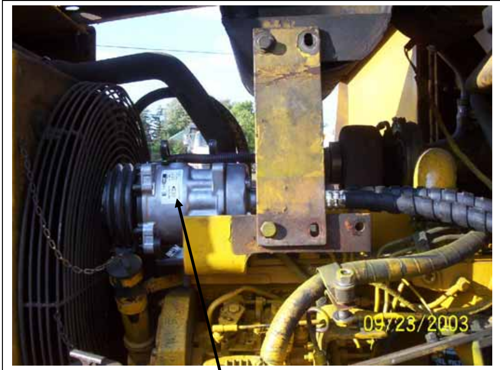
Compressor in place without 2 inch spacer
